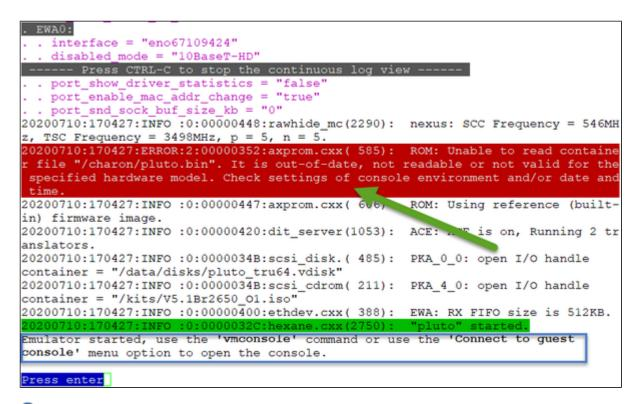
(?) The error message above (white/red) is expected the first time the virtual machine is started. It tells the .bin file does not exist as it is initialized when console parameters are set
