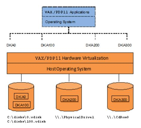
With the use of current storage technology, disks do not have to be physically attached to the Host platform, they can also reside on a SAN or iSCSI storage structure.
