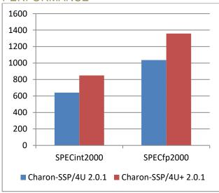
Single CPU test run on Charon-SSP/4U(+) with Solaris 10 on Intel  $6^{\rm th}$  gen CORE i7-6700 @ 4.0GHz CPU
