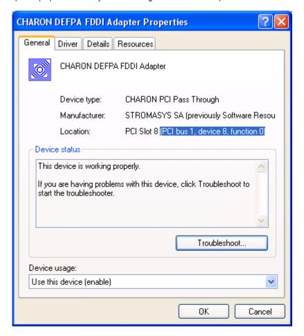
The "Location:" on the above picture gives X, Y, and Z for the "host\_bus\_location" parameter, for example:
