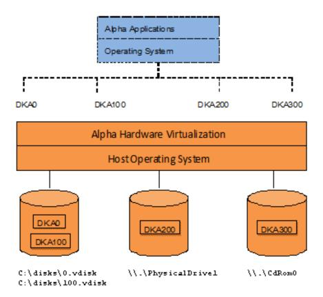
With the use of current storage technology, disks do not have to be physically attached to the Host platform, they can also reside on a SAN or iSCSI storage structure. A similar translation process is also valid for other emulated hardware devices.
