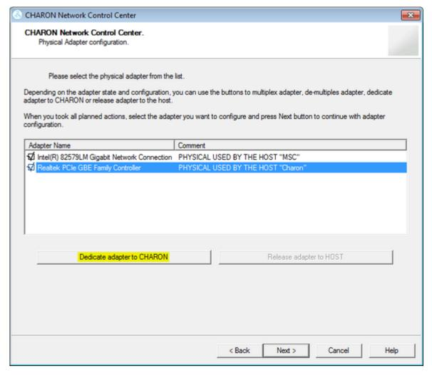
Install and configure VLAN adapters, according to the vendor's User's Guide, if required. Select the VLAN adapter in the dialog box in the above example. A VLAN adapter is not configured differently, the same procedure should be followed.
