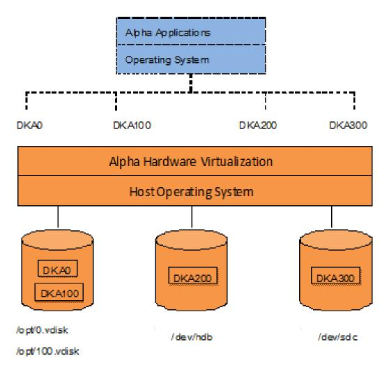
With the use of current storage technology, disks do not have to be physically attached to the Host platform, they can also reside on a SAN or iSCSI storage structure.
