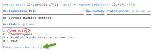
An AlphaServer 4100 (1) will be added by cloning the as4100 configuration file template (2 & 3) to the /charon/pluto.cfg (4 & 5):
