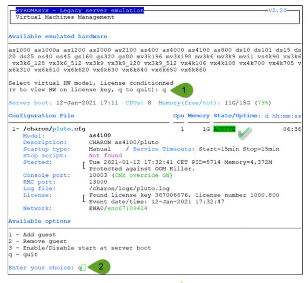
We can see below the service is active, meaning the emulator is running (1 this does not mean "booted") and will be automatically started at Linux server boot ("OnBoot" column on the right side)
