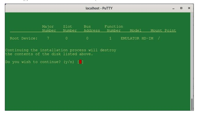
After the confirmation, the basic system with the essential operating system components will be installed and the system is automatically shut down.
